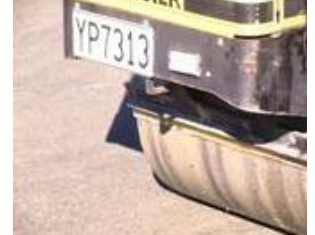
Vibrating roller compacts the crushed lime
